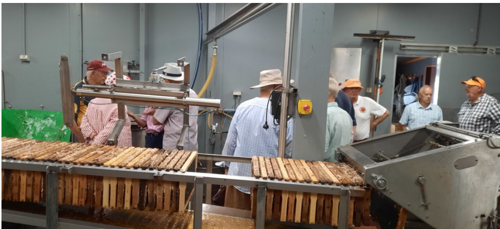
A long line of frames having the capping removed and heading to the spinner
