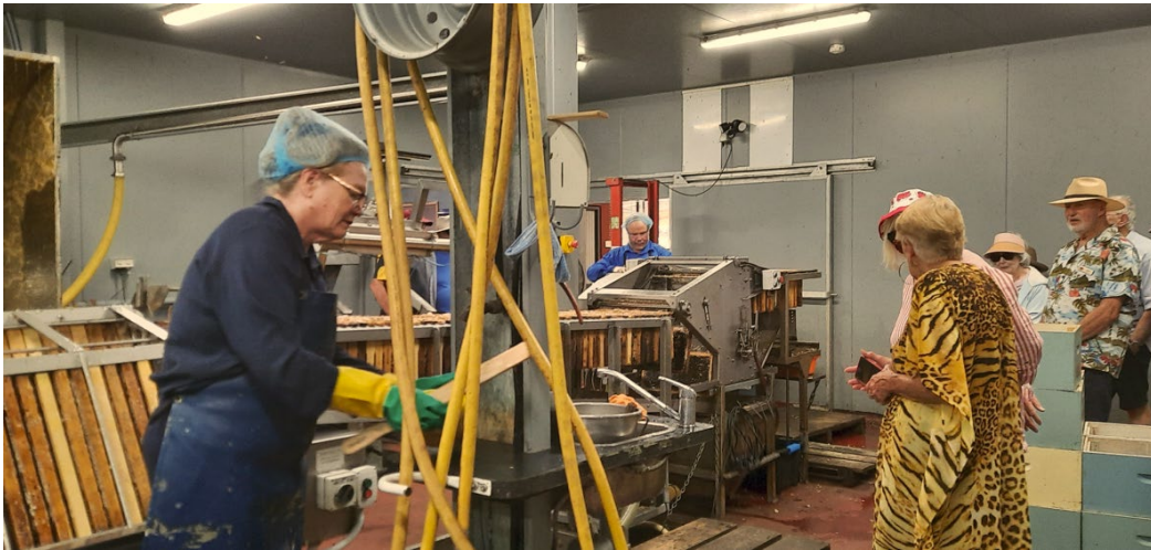
A long line of frames having the capping removed and heading to the spinner
