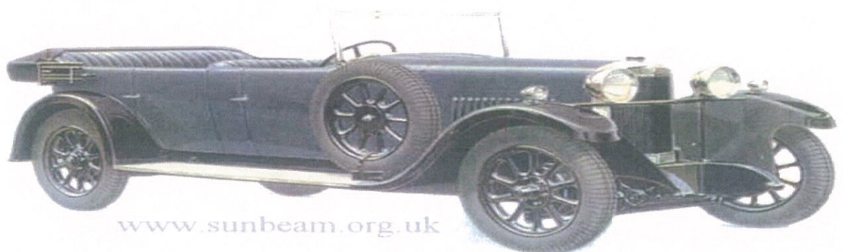
1929 Sunbeam 16hp This 2040cc 6 cylinder car was one of the most popular produced at Wolverhampton. It had a top speed of over 60mph and 4 wheel brakes were of course a standard fitment.
